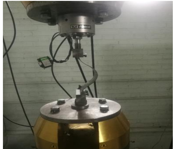
Fig. 2. Buckling of composite plate under pressure loading
