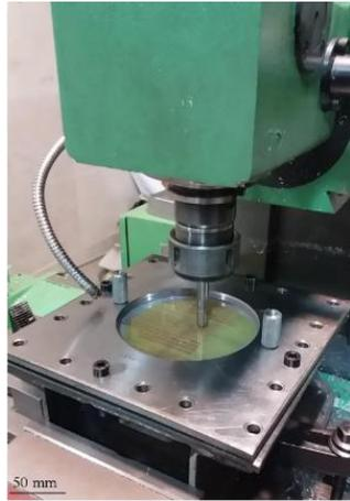
Fig. 1. Performing the SPIF process on a CNC milling machine.
