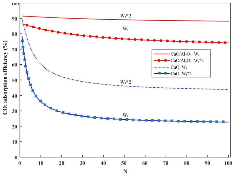
Fig. 1. Effect of the solids inventory on CO<sub>2</sub> adsorption efficiency achieved by CaO and CaO/Al<sub>2</sub>O<sub>3</sub> sorbents
