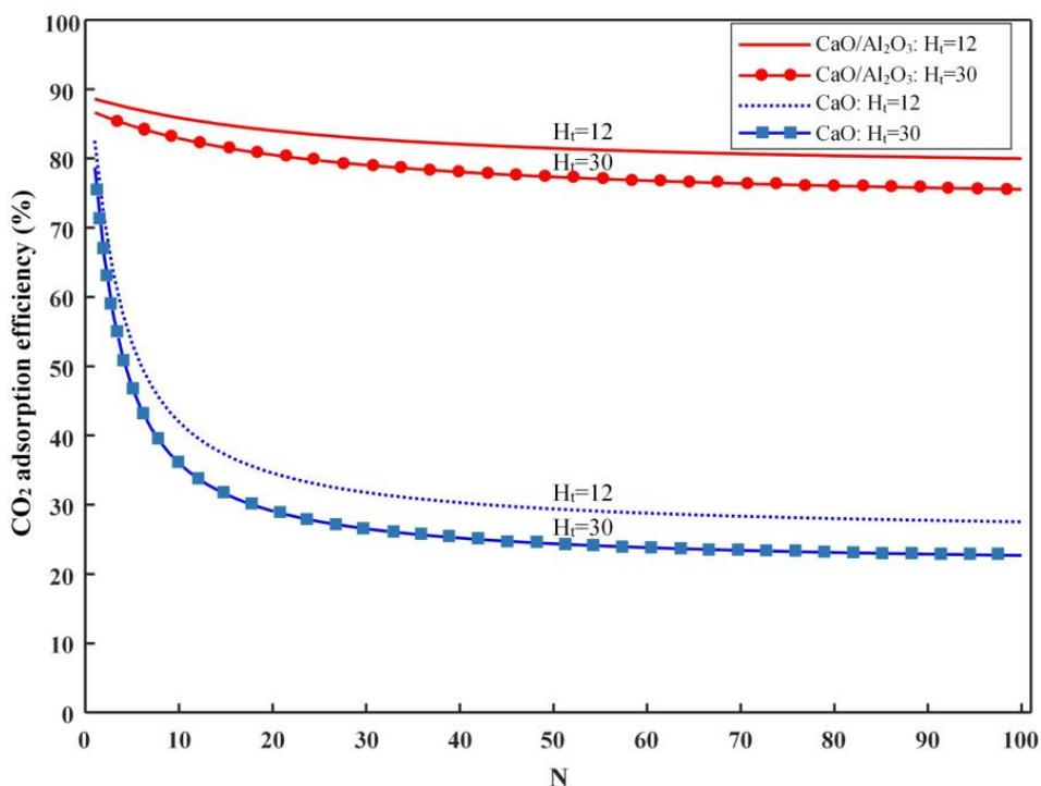
Fig. 3. Effect of total height of the carbonator on CO<sub>2</sub> adsorption efficiency achieved by CaO and CaO/Al<sub>2</sub>O<sub>3</sub> sorbents
