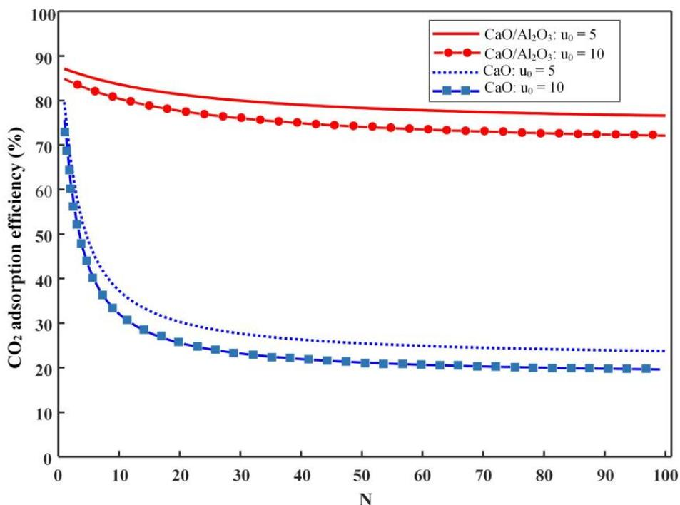
Fig. 2. Effect of the superficial gas velocity on CO<sub>2</sub> adsorption efficiency achieved by CaO and CaO/Al<sub>2</sub>O<sub>3</sub> sorbents
