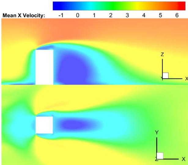
Fig. 3. Contour of mean X-Velocity in  $y=0$  plane (upper) and  $z=0.01\text{m}$  plane (lower)
