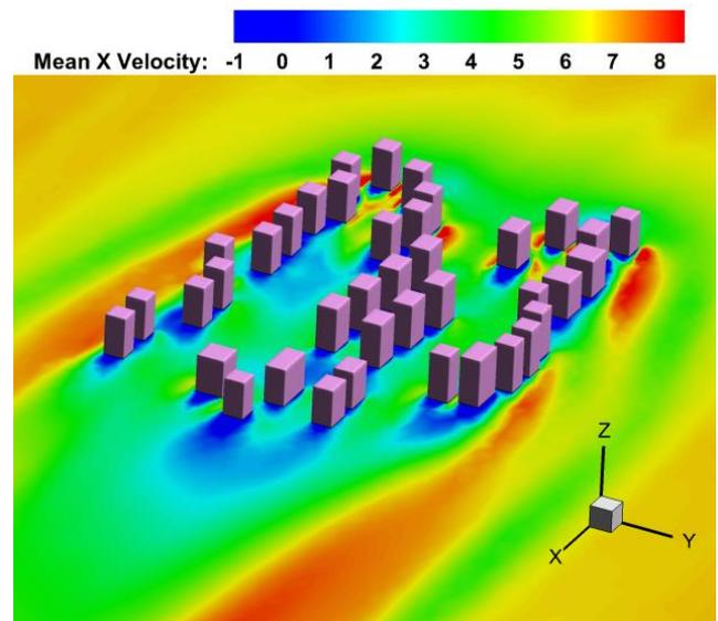
Fig. 4. Contour of mean X-velocity at  $z=1\text{cm}$  plane
