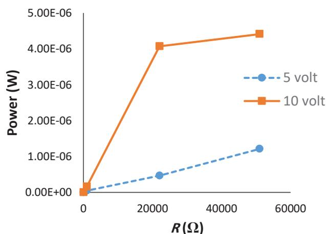
Fig. 4. The effects of external resistance on the power output (27 $\mu$ l, 6.5Hz)
