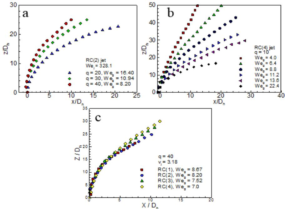
**Fig. 1. Trajectory results obtained for a) RC (2) at the momentum ratios 20, 30 and 40  $We_j=328.1$ . b) Effect of gas Weber number for RC (4) at momentum ratio of 10. c) Effect of aspect ratio for the momentum ratio of 40.**
