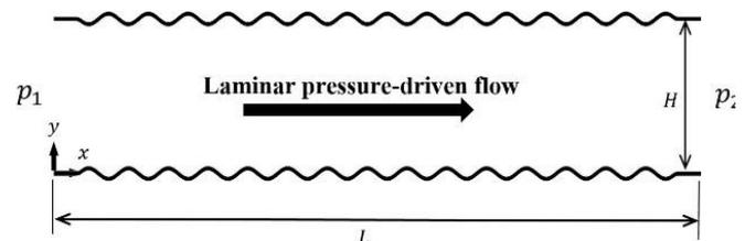
**Fig. 1. Schematic of a two-dimensional laminar pressure-driven flow within a microchannel with sinusoidal surface ruggednesses**
