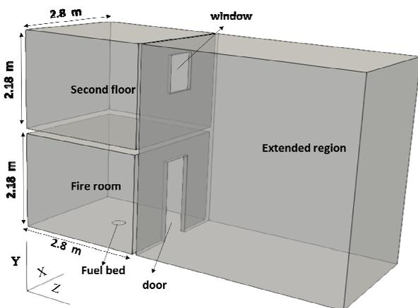
Fig. 1. test case of two-floor building
