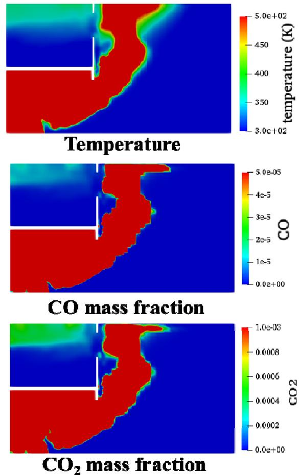
Fig. 2. Temperature field and toxic gases for a heat release rate of 5000 kW at 40s
