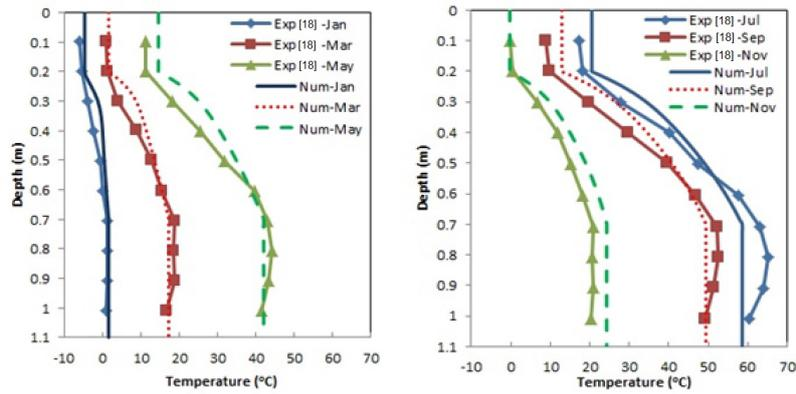
Fig. 4. Temperature distribution predicted by numerical simulation with measured data for cubic pond of Urmia
