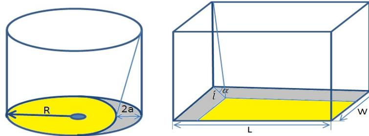
Fig. 1. Schematic of ponds with circular and rectangular cross-sections along with their shaded areas
