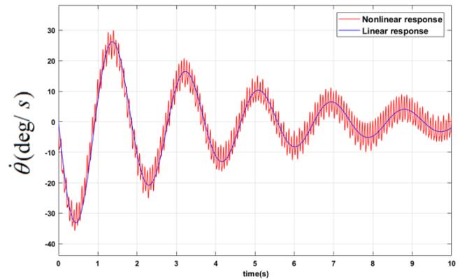
Fig. 3. Comparison of linear and nonlinear responses for pitch rate
