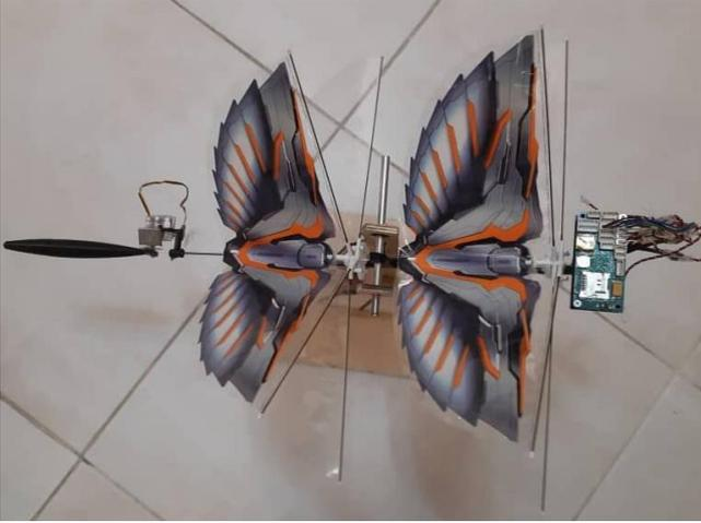
Fig. 1. The proposed dragonfly-like MAV with a new structure
