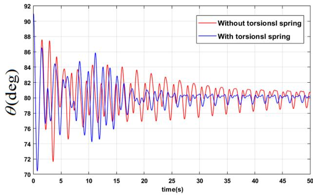
Fig. 4. The role of tail movement as a vibration absorber
