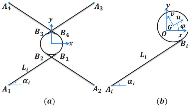
Fig. 1. 4RPR parallel planar manipulator (a) Schematic diagram of model (b) Kinematic configuration. ([6])
