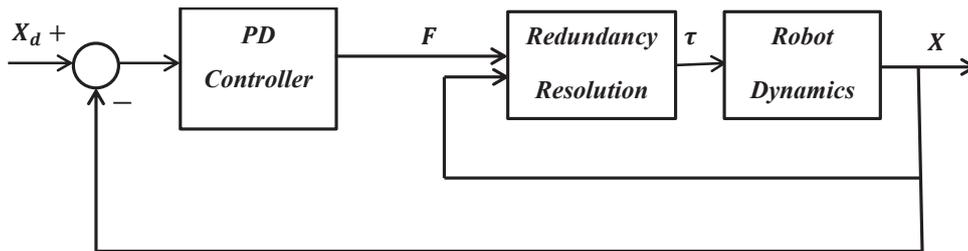
Fig. 2. Block diagram of the closed-loop control topology using an inverse dynamics control.
