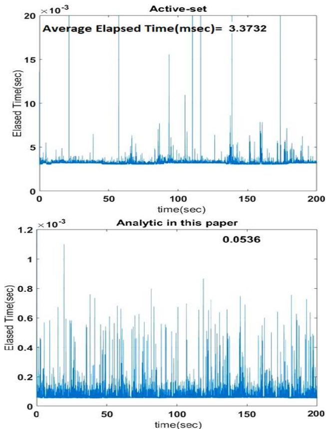
**Fig. 3. Total elapsed time to calculate optimal forces in circular path at analytic-iterative redundancy resolution.**
