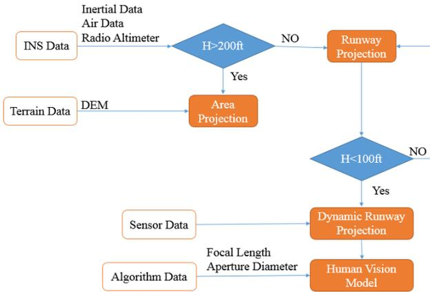
Fig. 1. Frame of proposed landing navigation
