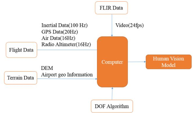
Fig. 3. Block diagram of the depth perception cue implement
