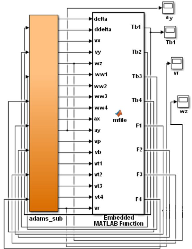
Fig. 1. Co-simulation model of combined control of chassis system
