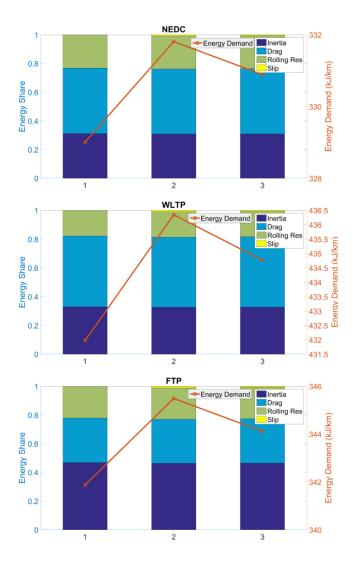
Fig. 2. Energy demand and share of each resistance for compact B-class sedan, 1: neglecting the slip loss, 2: considering the slip loss using physical tire model, and 3: considering the sip loss using verified tire model
