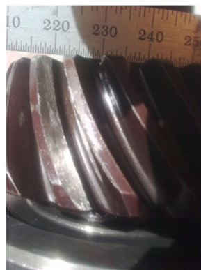
Fig. 2. (a) Faultless gear, (b) faulty gear with 20% wear, (c) faulty gear with 40% wear, (d) faulty gear with 60% wear
