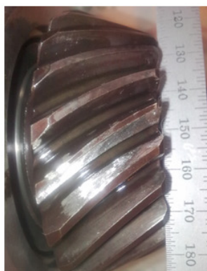
Fig. 2. (a) Faultless gear, (b) faulty gear with 20% wear, (c) faulty gear with 40% wear, (d) faulty gear with 60% wear
