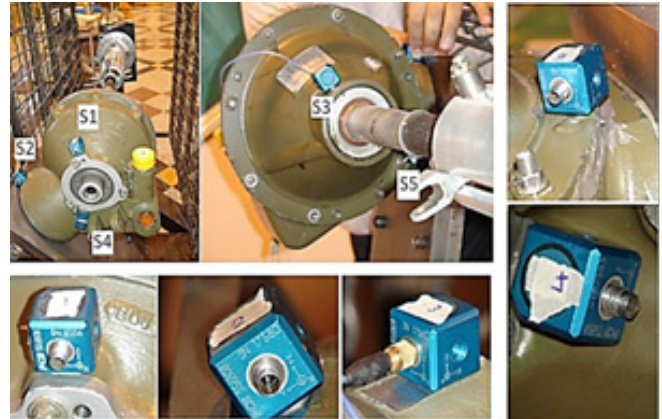
Fig. 3. Positions of tri-axial accelerometer sensors mounted on the tail gearbox
